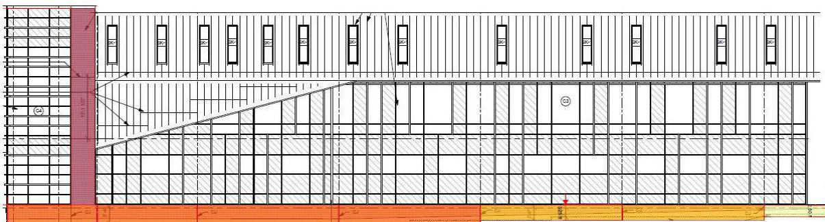
Figure 6.8: North Elevation Panel Breakdown. Image by George Andonie, modified from Sheet A3.1.1
